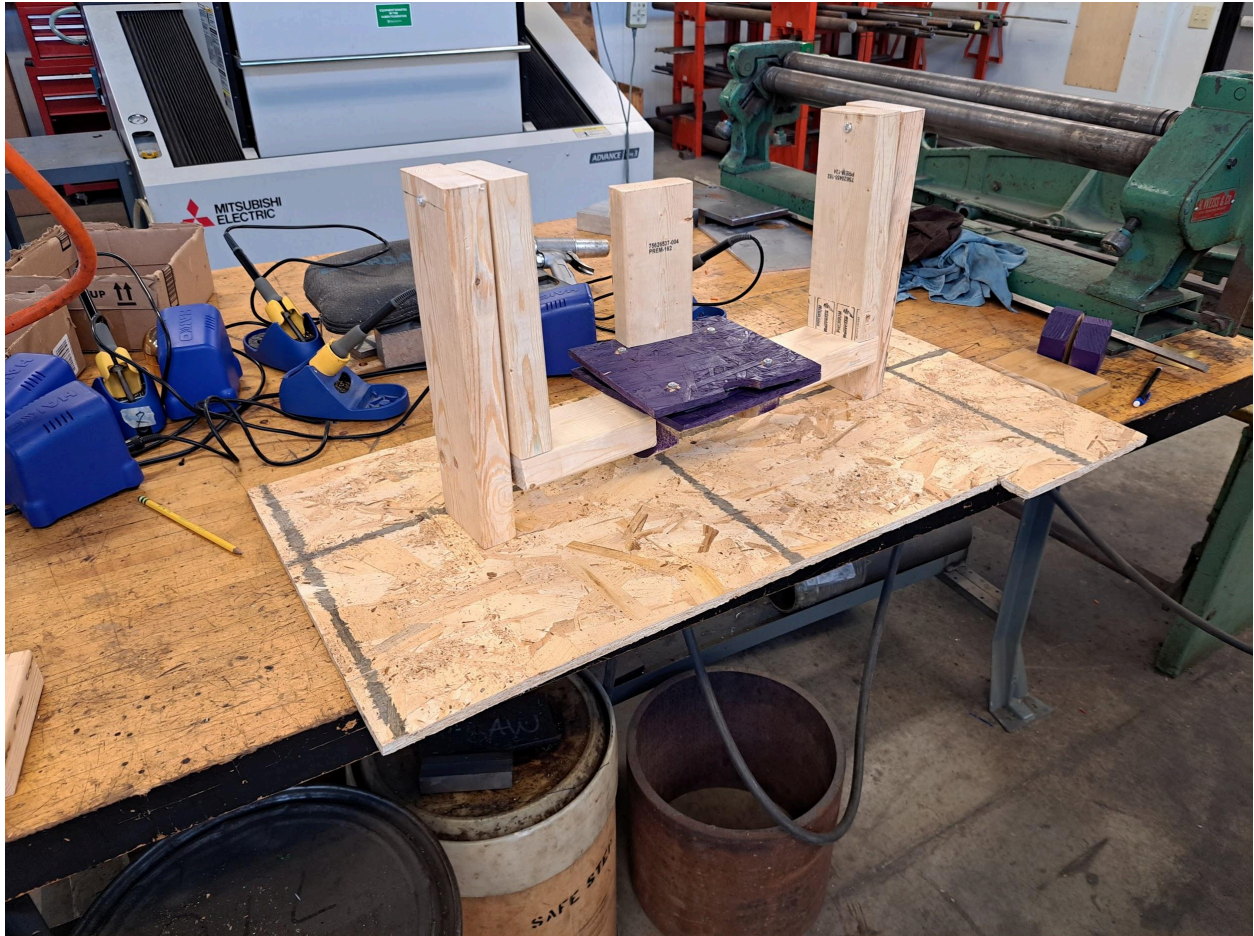
Figure 3.6.2.1: Initial wooden prototype of the Ball Spinner Mechanism
